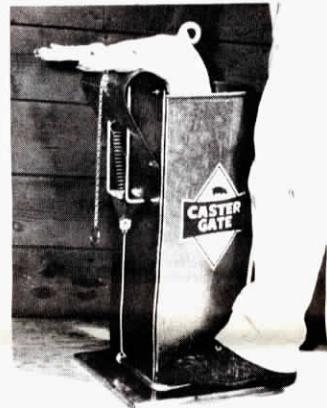
Foot-operated body band inside Caster Gate holds hog firmly but gently in either "up" or "down" position.
