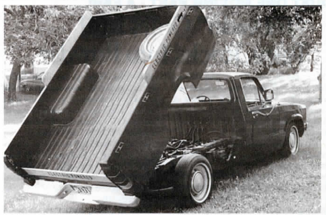
Batteries are mounted below hinged pickup bed, making them easy to get at for service and maintenance.
