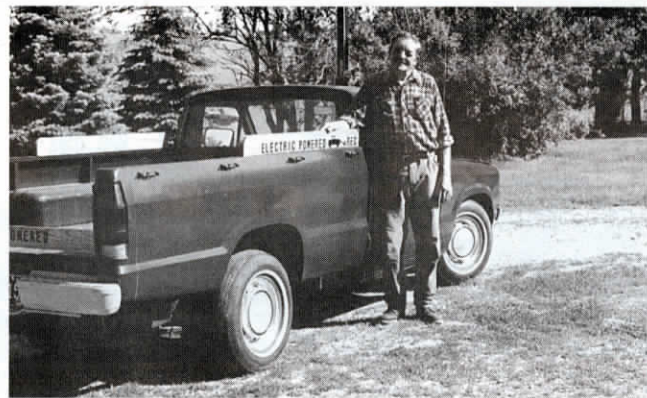
Dozler converted a 1981 Ford Courier with a blown 4-cyl. engine to an electric-powered rig. It's equipped with 20 Trojan 6-volt deep-cycle marine-type batteries.
