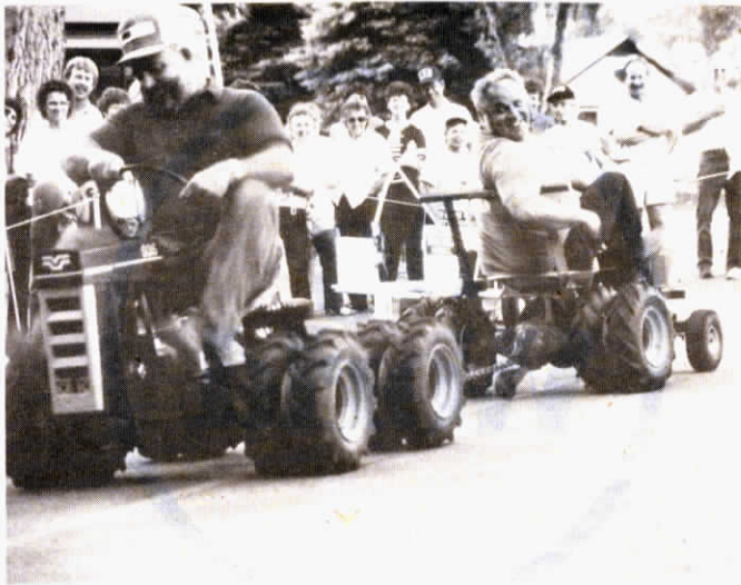
Built to stand up to adult abuse, 4-WD mini Versatile hinges in the center for steering and has duals all the way around, while 2-WD Deere replica has rear dual wheels.
