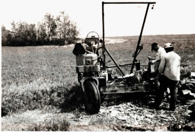
Overhead cylinder-operated boom maneuvers heavy pieces into position for splitting.
