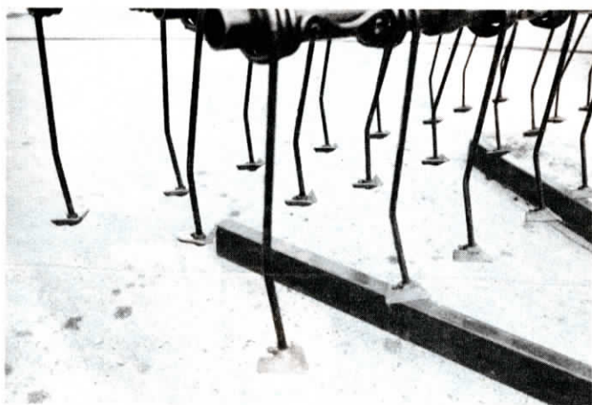
Mounted near the end of the tines, the cultivator "shoes" work almost as deep as the tines would normally go.
