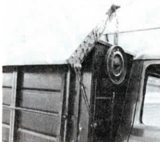
Two belt-driven 12-in. dia. pulleys (one on each side) open and close the two halves of the cover.
