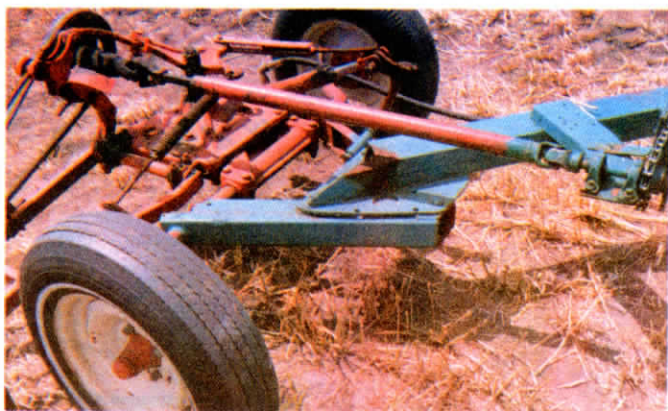
Home-built hitch lets Bertholet operate two IH 9-ft. sicklebar mowers at the same time behind his Massey Ferguson 35 tractor.
