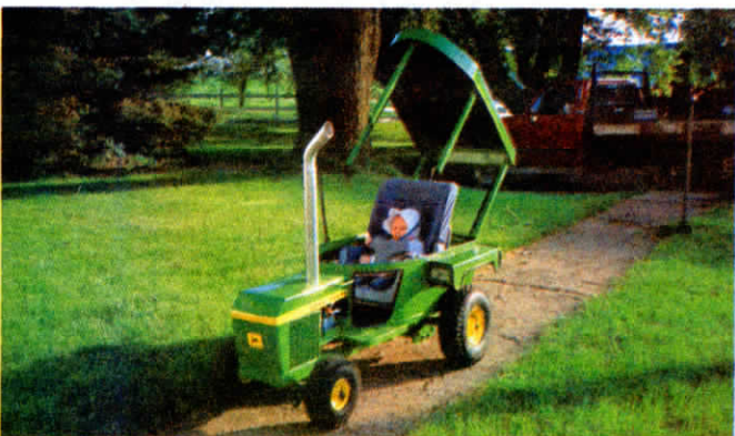
Cab is hinged at bottom to provide easy access to seat. Push handle mounts on back.
