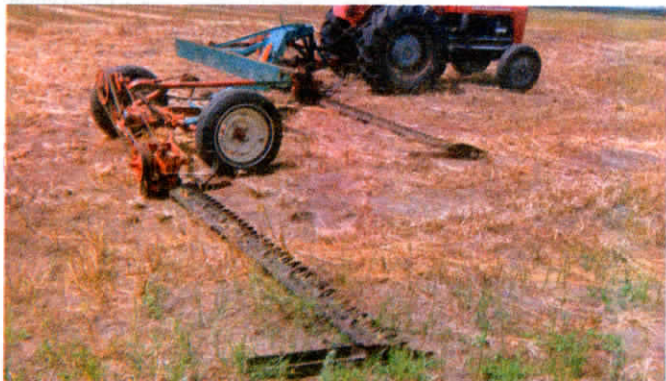
Steel frame hooks up to back mower, which is operated by chain-driven pto shaft.
