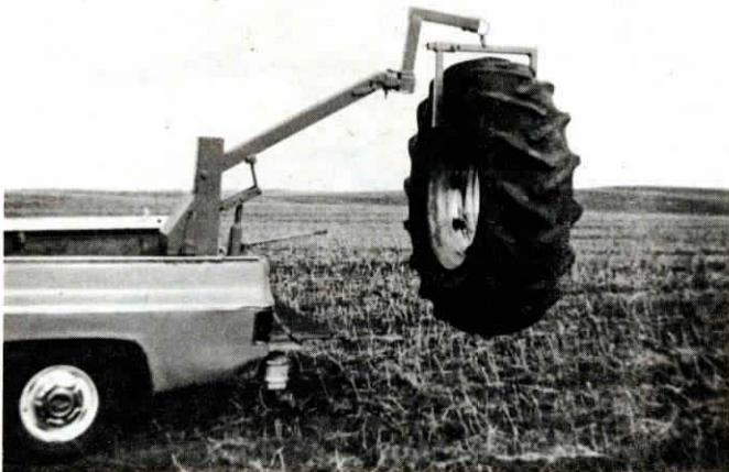
Boom also handles barrels, engines and other loads up to 800 lbs.
