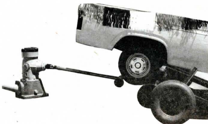
Power Pump uses 6-ft. driveshaft to power irrigation pump.
