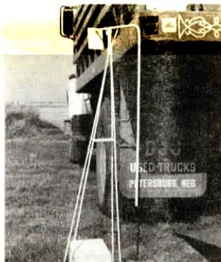
Truck rear corner bumps spring-loaded "flag" to signal correct position.
