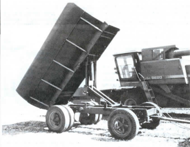
An 18-ton Low Boy hoist is used to dump wagon which rides on 20-in. wheels.
