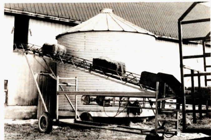
The bottom, horizontal elevator slides into hay rack as bales are unloaded.
