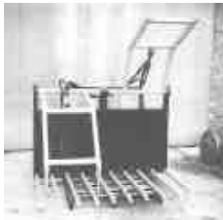
Each side of new grapple fork operates independently.
