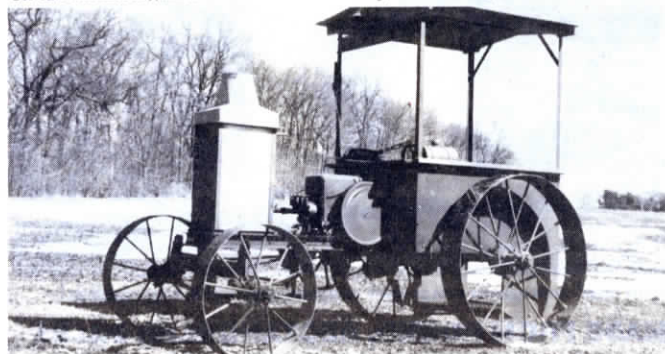
Tractor's steel wheels are from a horse-drawn manure spreader.
