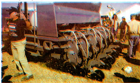
Row units are made out of 1-in. plate steel. All pivot points and wheels have Timken bearings. Solid steel press wheel is chain-driven.
