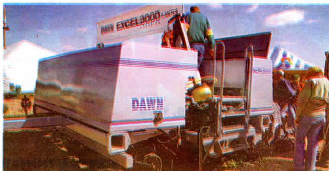
Dawn's row crop planter looks more like a big grain drill because it's fitted with big-capacity seed hoppers. Front fertilizer toolbar adjusts up and down hydraulically.
