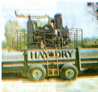
A 580 hp. diesel engine drives a 320 kw generator to provide electric power.
