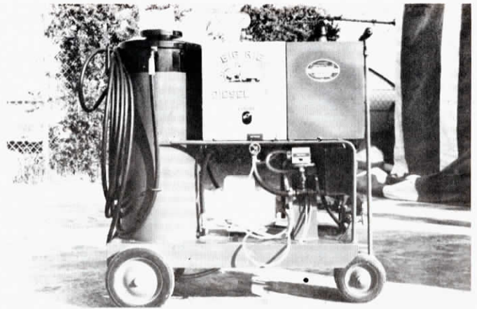
Big Red burns No. 2 diesel fuel.
