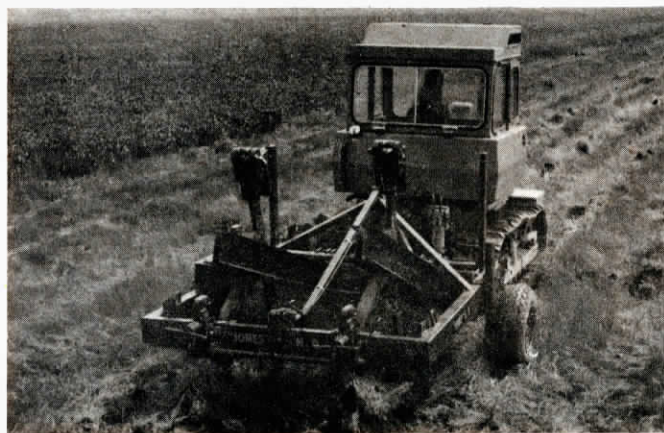
Spring-loaded I-beam instantly raises shank out of ground when a rock or other obstacle is struck.
