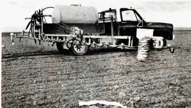
Weighted strips of paper fall from covered roll at end of boom.
