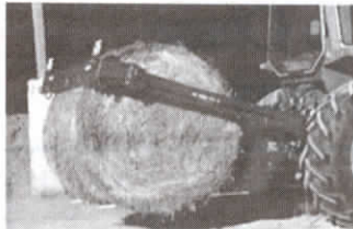
Bale is squeezed between bottom-mounted forks and sicklebar for transport. To cut the bale, you set it on the ground and lower the sicklebar into it.
