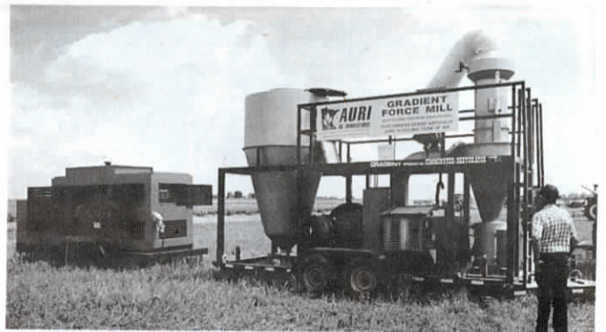
This pre-production prototype mounts on a flatbed and is powered by a 100 hp. electric motor. Grain or other materials are loaded into the funnel at left and processed in the funnel at right.
