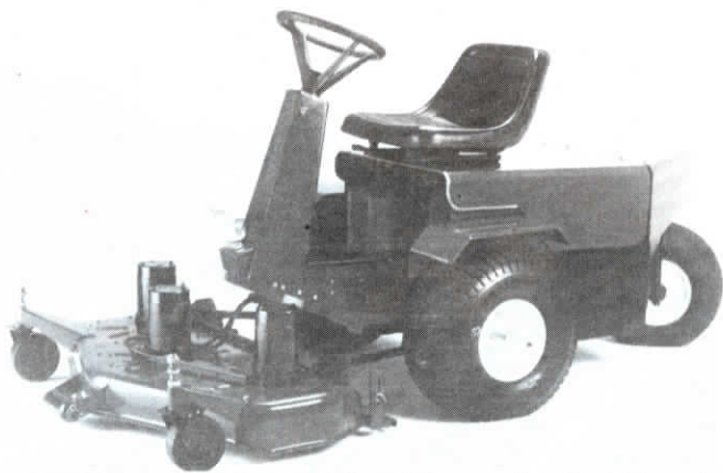
Turf Star 2000 uses six 6-volt deep cycle batteries to power three direct-drive motors mounted on top of mower's 3-blade, 44-in. deck.
