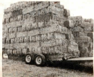
Self-unloading wagon drops to ground for unloading.
