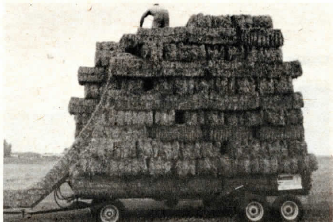
"Pusher chute" self-loads bales from baler onto tag-along trailer.
