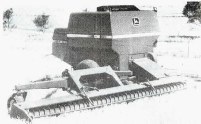
Front of the new 1051 is permanently mounted on a two-wheeled cart.
