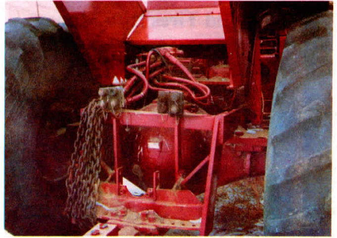
Tractor's Clarke planetary rear axles and transfer case are the type used on big earth moving and logging trucks.
