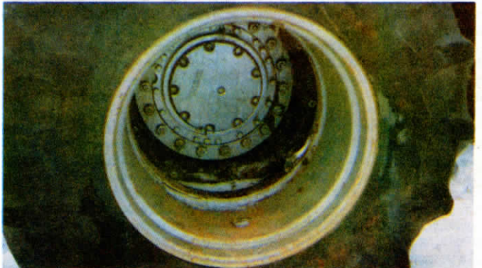
Above photo was taken with duals mounted on the tractor. Laughlin moved the inside wheel rim in 6 in. and welded it to the axle, then moved the outside wheel rim out 9 in. in order to get the proper wheel spacing.
