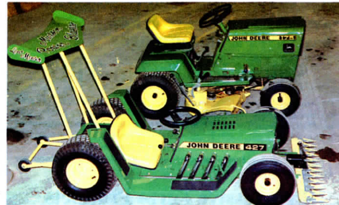
Madson built "dragster" mower in foreground out of two junked Deere 175 riding mowers similar to one in background.
