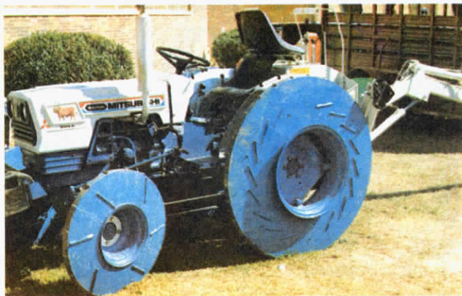
Anderson mounts a smaller steel wheel in front. It spins faster than the rear, helping pull the tractor ahead in mud.
