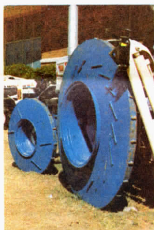
Steel mud wheels narrow to a slim 1 1/2 in. tread that cuts forward resistance.
