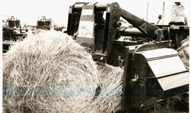
Cutter knife along lower edge of rear lift gate cuts through big bale, or silage, and pulls material into hopper. Feeds out the side into bunks or onto ground.
