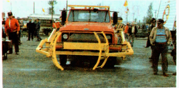
Bale Boss picks up bale in front and loads it on bale rack at rear.
