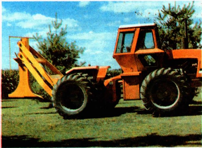
Tiler uses a chain depth guide to maintain grade. In most soils, one tractor is enough to pull it.
