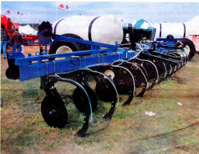
An "in between" caddy can be used to pull Progressive Farm Products' strip-till applicator, which consists of a 20-in. coulters followed by anhydrous knives and disc sealers (not shown in photo).
