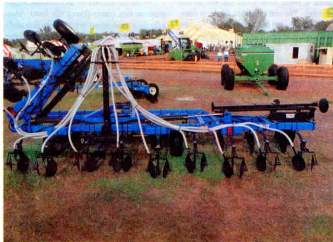
DMI builds both pull-type and mounted strip-till applicators. Disc sealers leave a mound of soil that the company says warms up faster than a bare strip in the spring.
