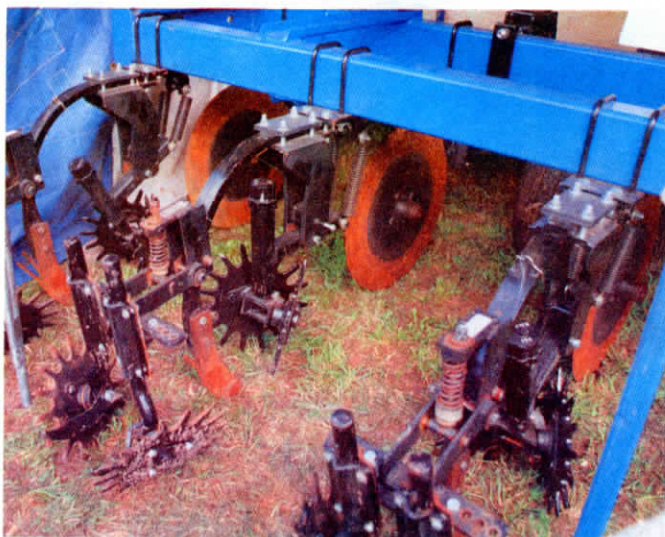
You can turn any fertilizer applicator into a strip-till machine using Dawn's Trashwheels and the company's new Trashhandler spiked closing wheels.
