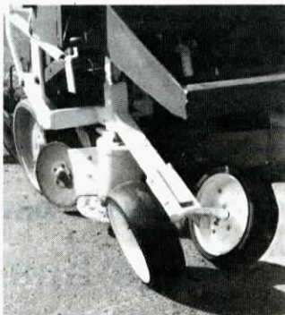
Angled "bogie" wheels follow ridge contour while disc behind shears off top of ridge, just ahead of planter unit.
