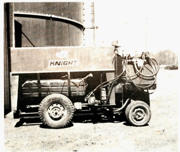
A front-wheel drive car engine and transmission power the mixer-feeder.
