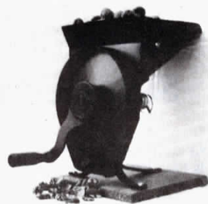
A hand-cranked "whacker" does the cracking on the Davebilt nutcracker.
