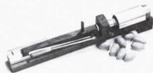
Rubber bands pull piston-type knocker into nut to shatter shell, but leave nutmeat intact.
