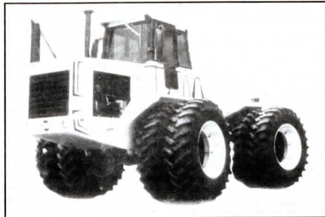
New CBT tractor has a Cummins engine, an Eaton transmission and differential, a Dana Clutch, and Muller axles.
