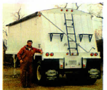
Cross pulls the trailer, which weighs 10,000 lbs., with a Ford semi tractor. He made his own Shur-Loc type tarp.
