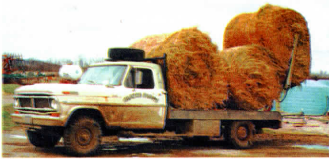
Garton can haul 3 big bales on extended pickup bed fitted with bale arms.
