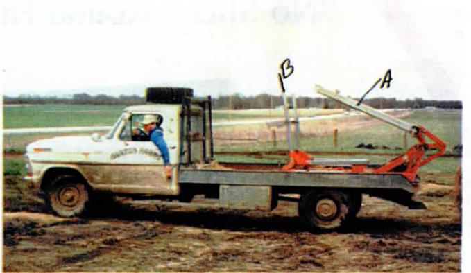
Crankshaft-driven hydraulic pump provides hydraulic power. Note bale arms at rear (A) and bale cradle at center (B).
