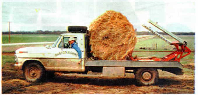
Bale handler drops first bale onto home-built cradle mounted at middle of bed. Cradle is rocked forward by hydraulic cylinders so bale rides just behind cab.
