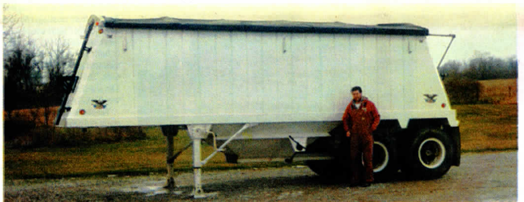
Cross built his own 24-ft. bottom-unload grain trailer for less than $5,000, using tandem axles for a better ride across fields.
