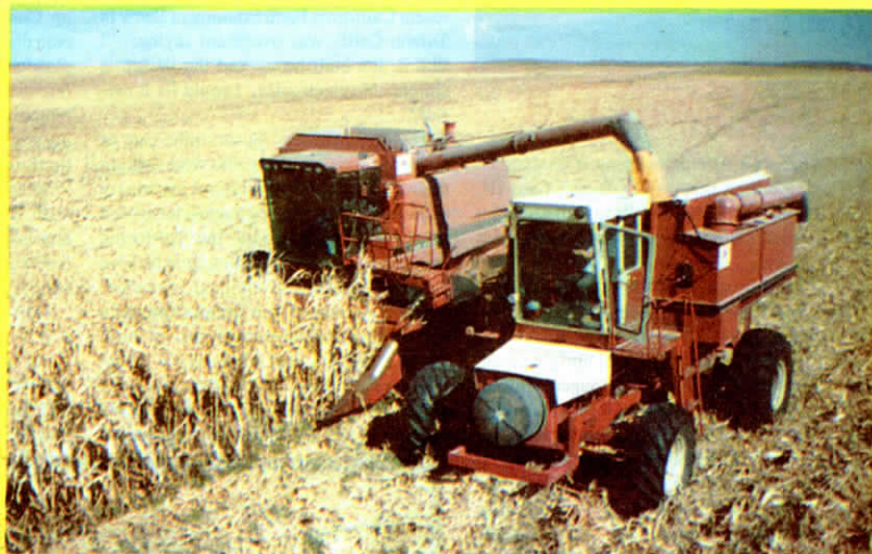
The Van Gieson's reversed direction of an IH 915 and mounted a 550-bu. hopper over the drive wheels to create an easy-to-handle, self-propelled grain cart.
