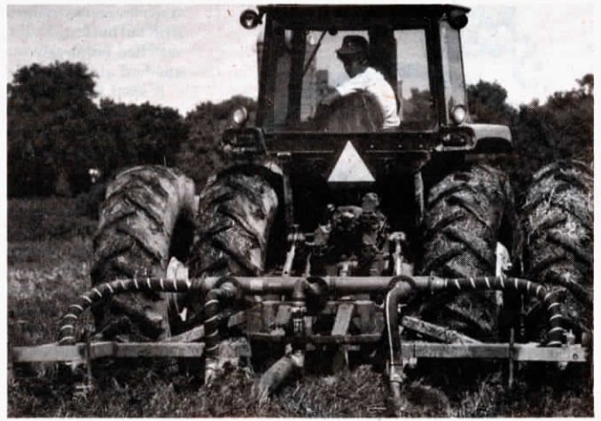
A long hose (a mile or more in length) links chisel plow directly to slurry tank or pit for injecting manure into ground without having to do any hauling.
