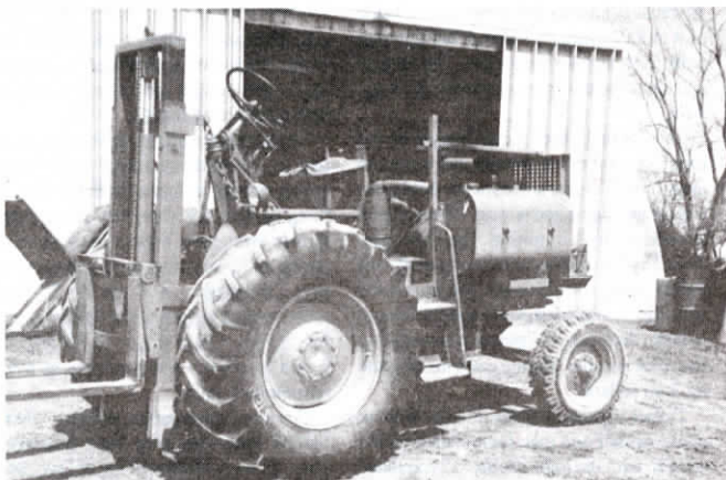
Van Den Brink made forklift out of two junked Deere 45 combines and other parts.
