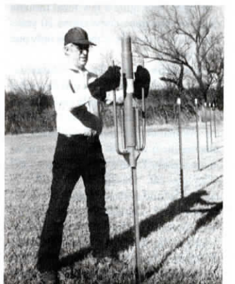
When the springs pull the outer shell back up, it slams against the head, lifting the whole driver for the next blow.
