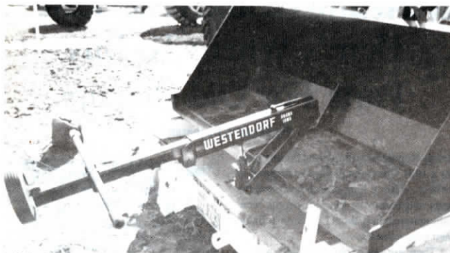
A 10-in. dia. rubber wheel at end of the extendable arm picks up the dual by the rim.
