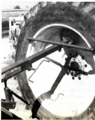
Hand crank moves arm in and out and a hydraulic jack raises and lowers the arm.
