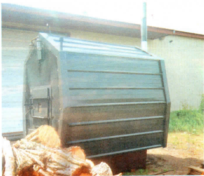
Elliptical shape of furnace and domed end sections help reduce stress on welds.
