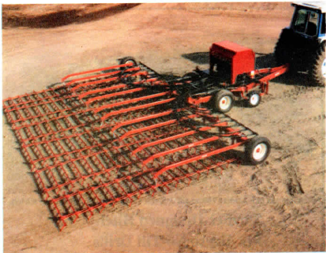
Gandy seed blower mounts on tongue of McFarlane harrow cart. Tubes run back to row of special brackets mounted across front of harrow.
