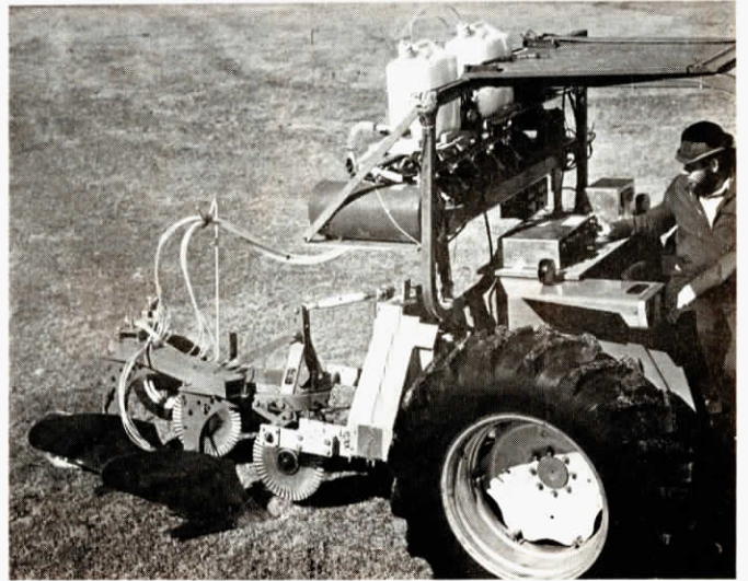
Nalco lubricant improved scouring and reduced draft up to 35% in NTML tests at Auburn, Ala. Test facility shown is much more elaborate than simplified kit developed by Nalco.
