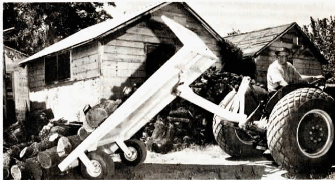
Trailer's unique hookup allows it to be dumped at any angle up to 45°, using the tractor's 3 pt. hitch.
