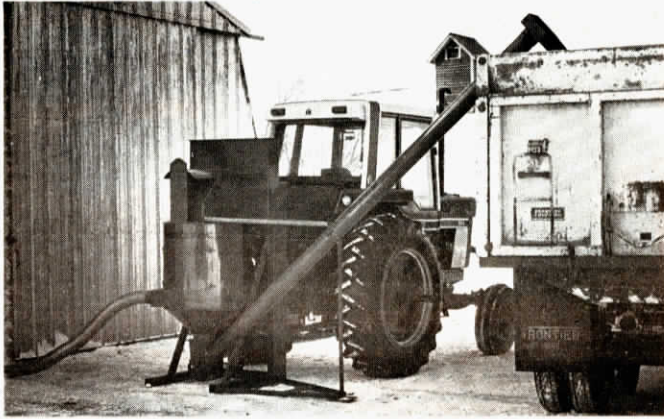
Vac-U-Loader's maximum capacity is up to 550 bu. per hr.
