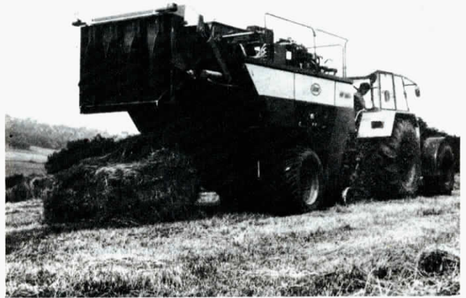
Vicon's new baler ejects its square bales "on-the-go".
