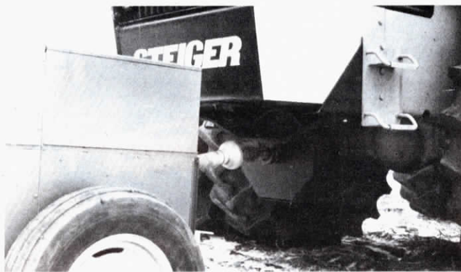
Front mounted pto for 4-wheel drives is powered off the tractor's crankshaft.
