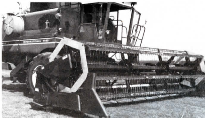
Photo shows reel expanded to 60-in. diameter from the standard 42 in.
