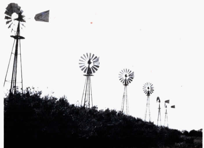
On a windy day, the six windmills pump about 3,000 gals. in 24 hrs.
