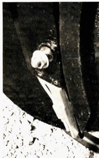
Metal "Fertle V" tube holder mounts in front of seed tube.
