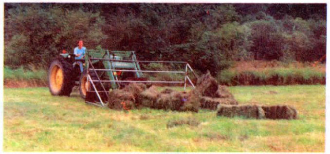
Big loader-mounted bale scoop picks up 10 to 20 bales at a time in the field.
