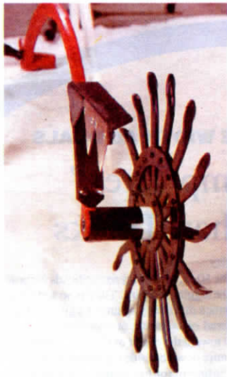
Kit consists of a pair of sickle blades that mount on rotary hoe arm and an axle extension with bearing protector that moves wheel over for extra clearance.
