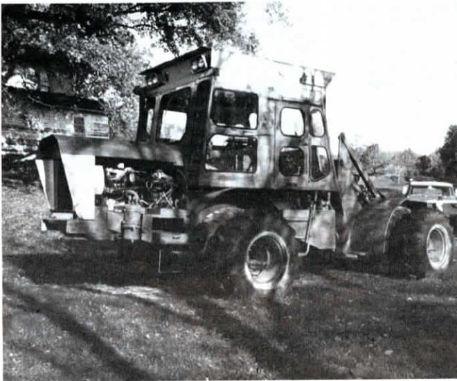
When Langerman put his tractor together, he wanted a cab big enough to walk around in and that would let him sit sideways while operating it.
