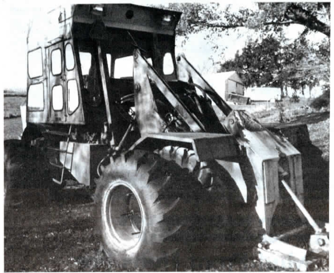
A 3-pt. hitch built onto the loader arms can be raised up out of the way to allow pull-type implements to be hooked up to tractor's swinging drawbar.
