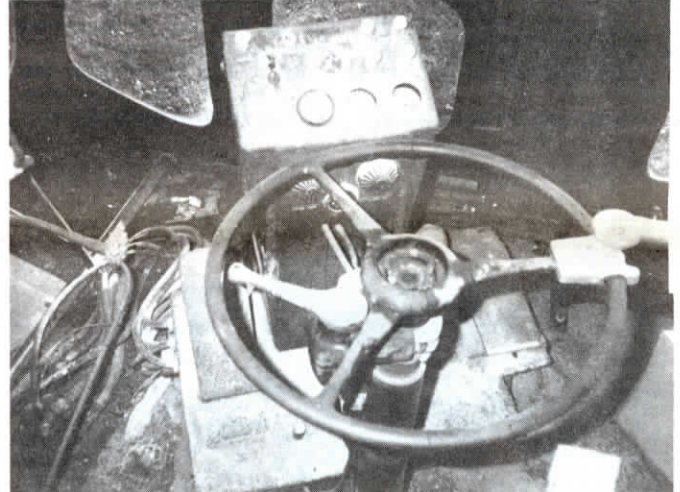
Lever under steering wheel is a hand clutch that Langerman uses instead of the foot clutch when he's hooking up implements and needs to "inch" along.
