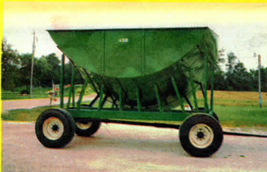
Semi-circular shaped steel box slopes down to one side (top). Outside of box is supported by 20 angle iron braces welded to wagon frame.
