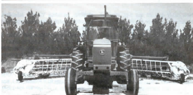
Walterscheids mounted a pair of side delivery rakes on a 3-pt. frame.
