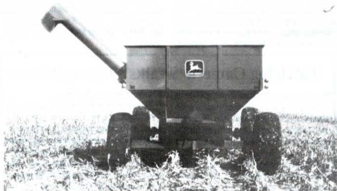
Harold Walters and Kenton Woster added a 2-ft. chunk to the axle of their new grain cart so it would match their 36-in. rows and follow in the tracks of their combine.
