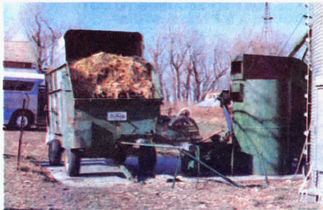
Production has already begun on the new residue burner. Electric motor automatically unloads crop residue into it from self-unloading forage wagons.
