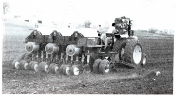
Calmer used parts from three 8-row IH 400 air planters to build innovative rig.
