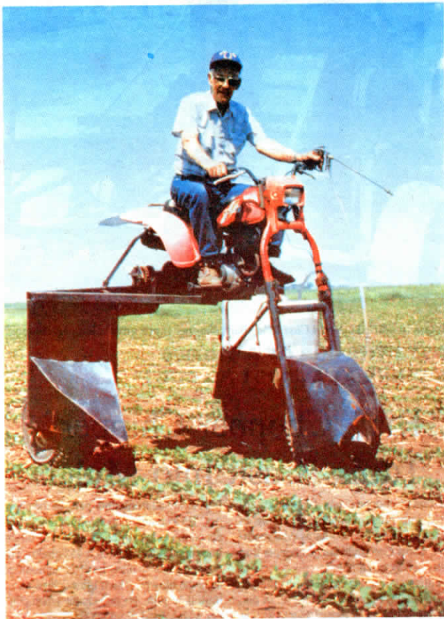
Jorgenson raised his 3-wheeler up 3 1/2 ft. and widened the rear wheels to 5 1/2 ft.
