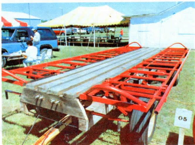
Moveable sides of new trailer drop down to unload bales or raise up to hold bales in place for transport. They also "open up" from the inside out to create a bale feeder.
