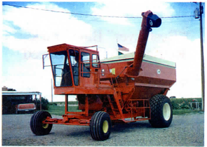
Grant built the grain hauler around a 750-bu. J&M pull-type grain cart. It’s powered by a Perkins 540 cu. in. V-8 diesel out of a Massey 760 combine.
