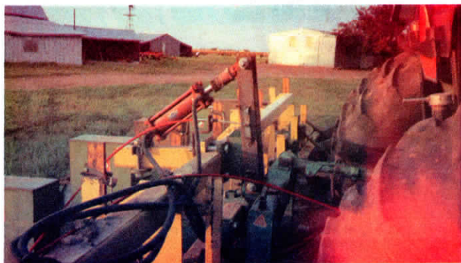
A lift bar attaches to 3-pt. top link and connects to a 4 by 8-in. cylinder. Steel cable, which runs to indicator ahead of cab, attaches to lift bar.
