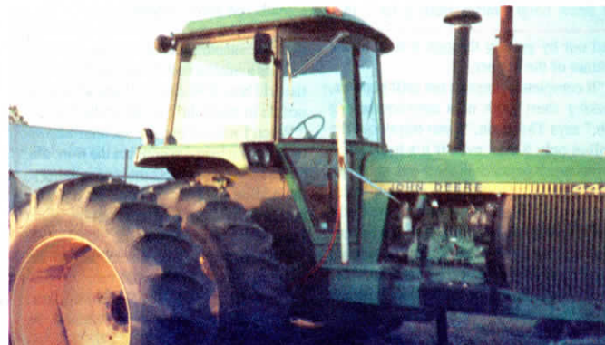
Indicator bar mounts on top of battery box at front right corner of cab.
