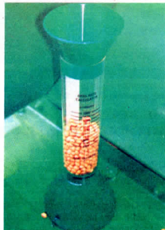
New drill calibrator is placed on top of any seed cup inside drill hopper and filled with a measured amount of seed.
