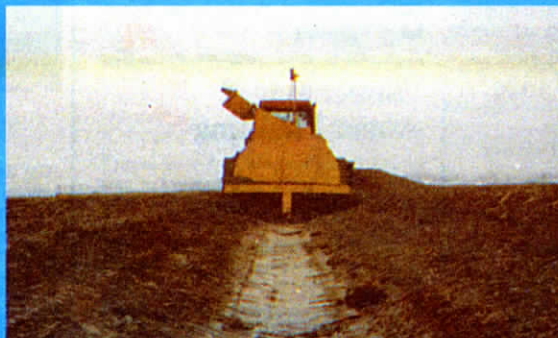
Junior Liebrecht's new ditcher consists of an 8-ft. dia. wheel that mounts on a tractor 3-pt. It flings dirt out as far as 120 ft. or it can dump dirt right alongside ditch.
