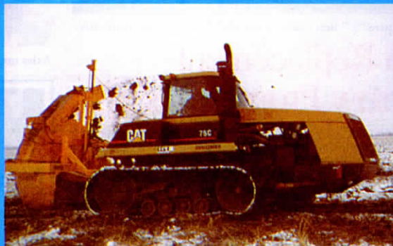
Junior Liebrecht's new ditcher consists of an 8-ft. dia. wheel that mounts on a tractor 3-pt. It flings dirt out as far as 120 ft. or it can dump dirt right alongside ditch.
